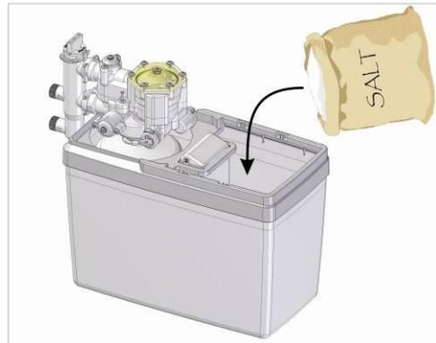
**5.3.** Add water in the salt bin until the water level is approx. 10cm (4") high. (the floater on the brine valve must be afloat)
