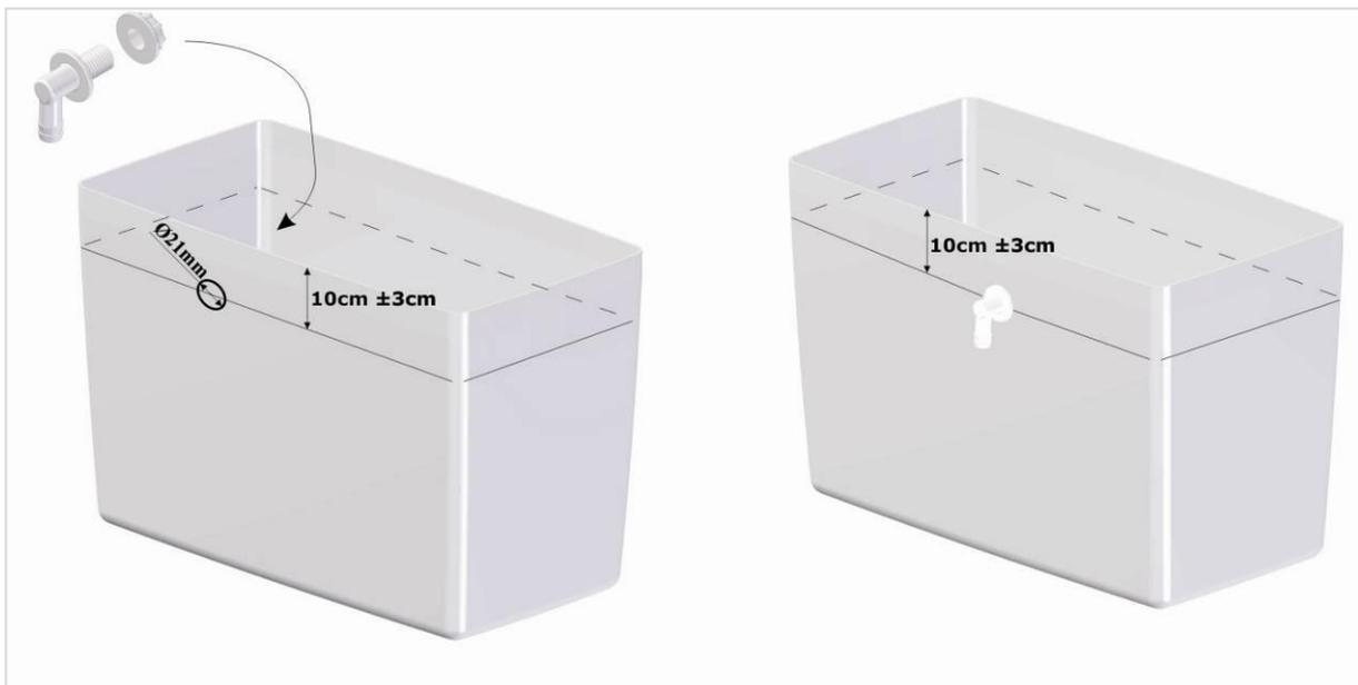
**3.3** Place the softener in the salt bin; use the side with the round opening (for correct installation, see 3.4). To install the brine valve, open the cover by pressing it gently at both sides. Now put the brine valve in the provided space, with the top side up. Make sure that the brine valve goes all the way down to the bottom of the salt bin. Make sure not to squeeze the tube; avoid kinks. Disconnect if necessary, and reconnect correctly. Close the cover.
